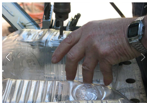
2. Holes are drilled in all sides of the juice containers, including the large one.
