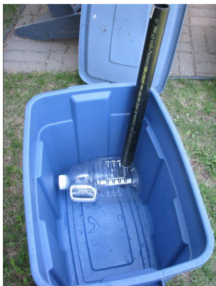
1. Recycled bins, abs pipe and juice bottles. Pipe is cut at an angle on the bottom and inserted in the large juice bottle
